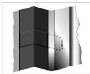
Figure 6: Raccordement vertical
